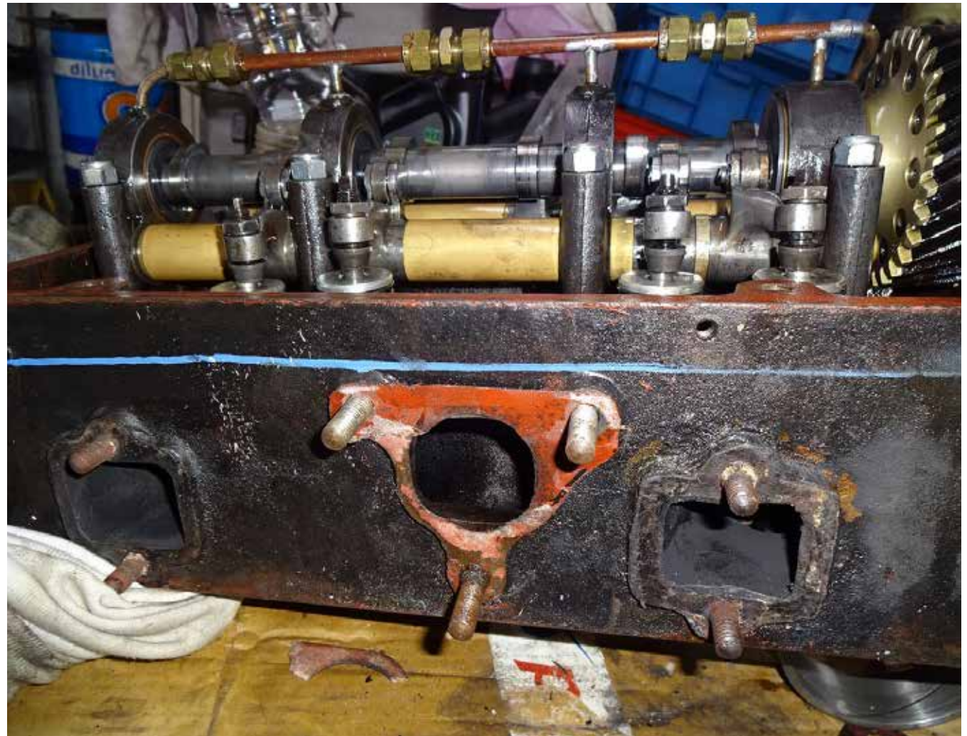
Photo 73: The cylinder head of the Lancia Lambda developed by Bob West in the 1940s
