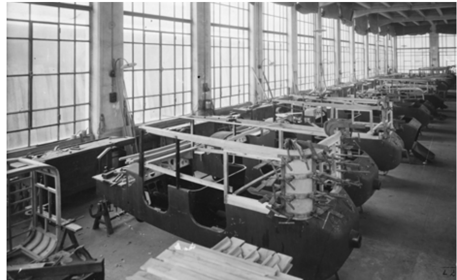
Photo 23: Assembly of the 'ballon' for the Lambda Torpedo
