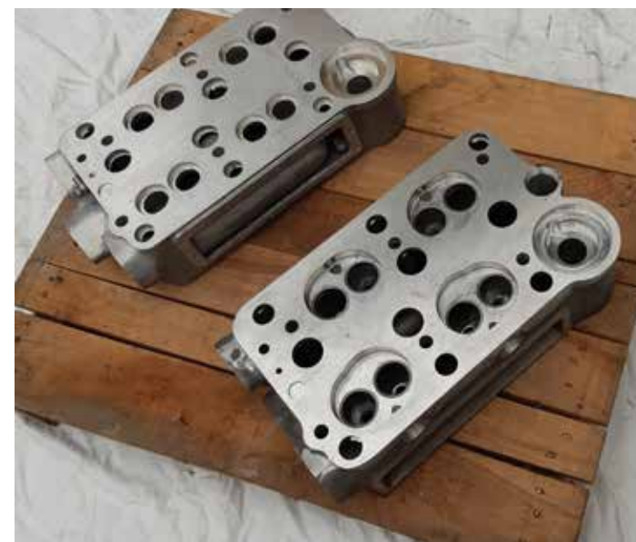
Photo 87: Lancia Lambda cylinder heads (left of early series, right of later series)
