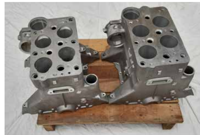
Photo 86: Lancia Lambda cylinder blocks (left of early series, right of later series)
